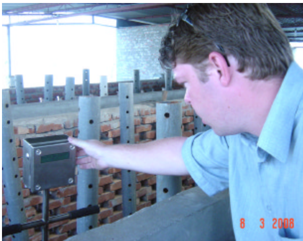
Oxygen level regularly monitored during the aerobic composting process
